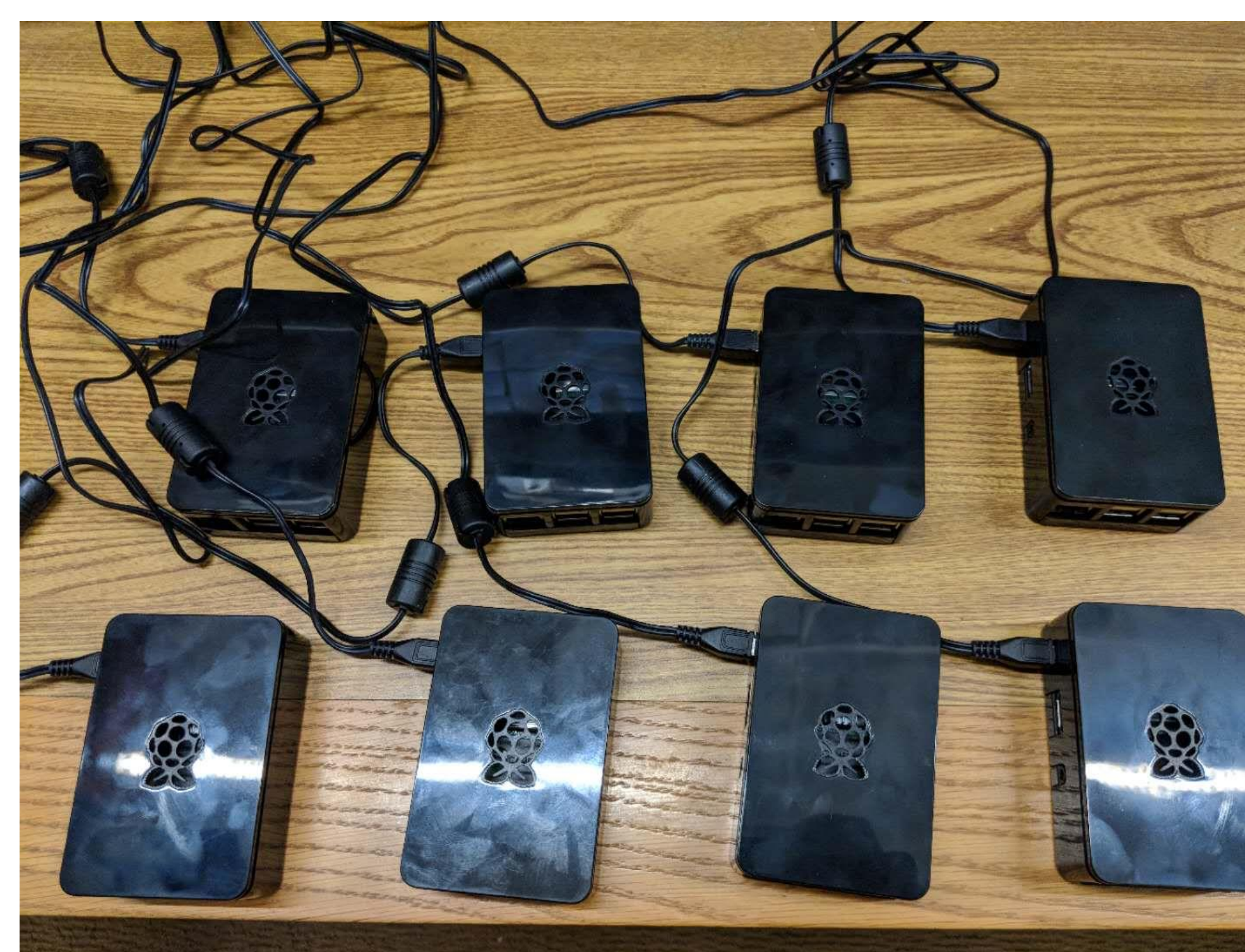
Figure 3. Edge Machine Learning System of 8 Raspberry Pis
