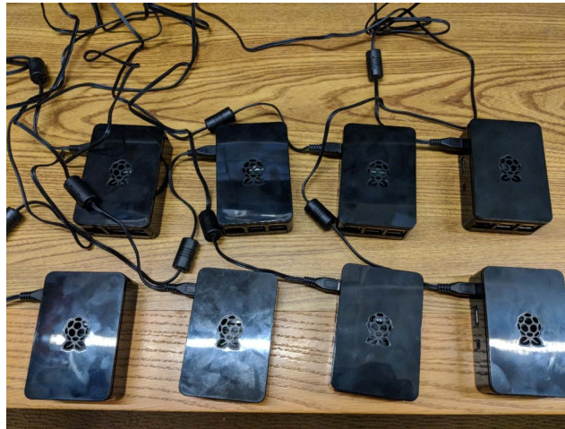
Figure 6: Edge Machine Learning System of 8 Raspberry Pis
